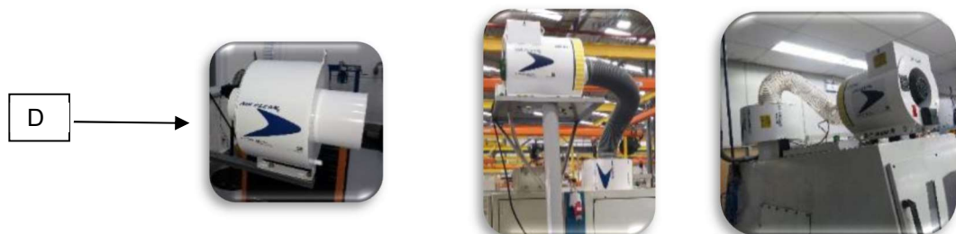
TYPICAL APPLICATION OF THE PREFILTER VERTICALLY.
